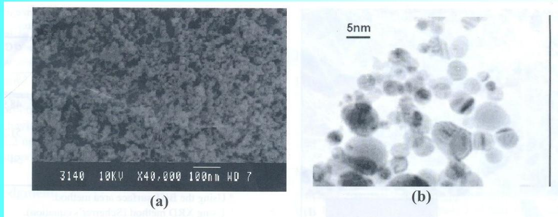
**(a) SEM image of MgO nanoparticles (b) TEM image of MgO nanoparticles.**
